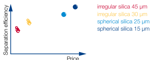
Comparison of separation efficiency and price of irregular versus spherical silica
